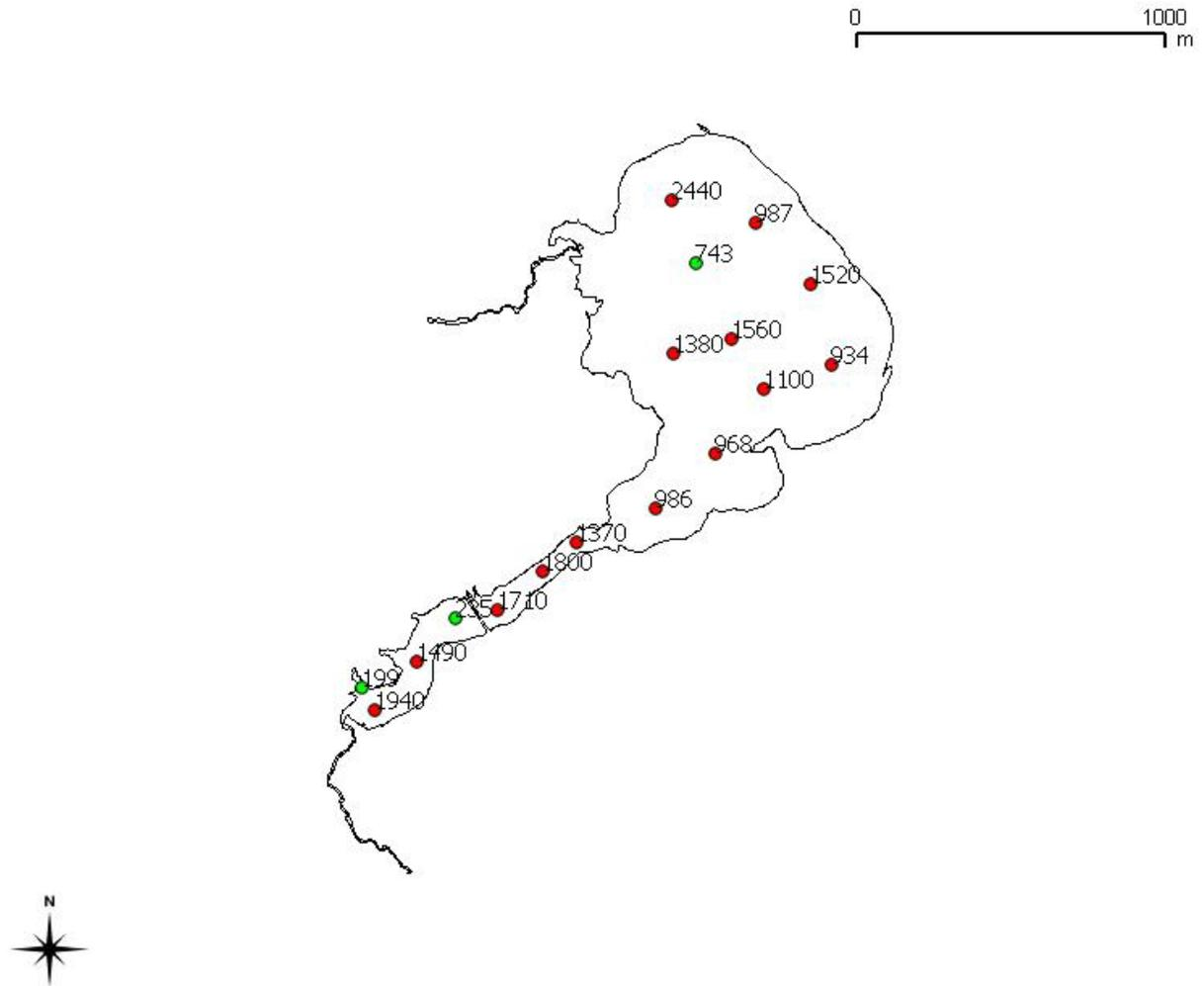
**Figure 8.** Total phosphate in Irishtown Reservoir in October 2009. Concentrations are in  $\mu\text{g/L}$ . Values in red are in excess of 900 in  $\mu\text{g/L}$  and are taken as indicative of eutrophic conditions.
