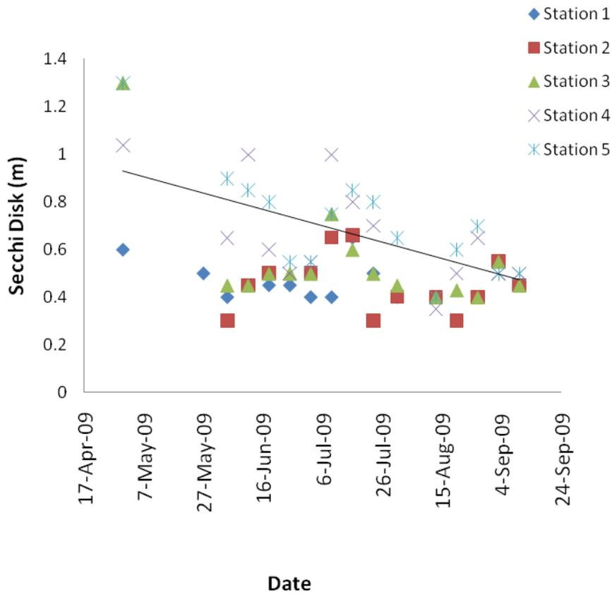
**Figure 4.** Secchi disk readings at the 5 sampling stations in Irishtown Reservoir in 2009. The line indicates a tendency to less light penetration as summer progressed.
