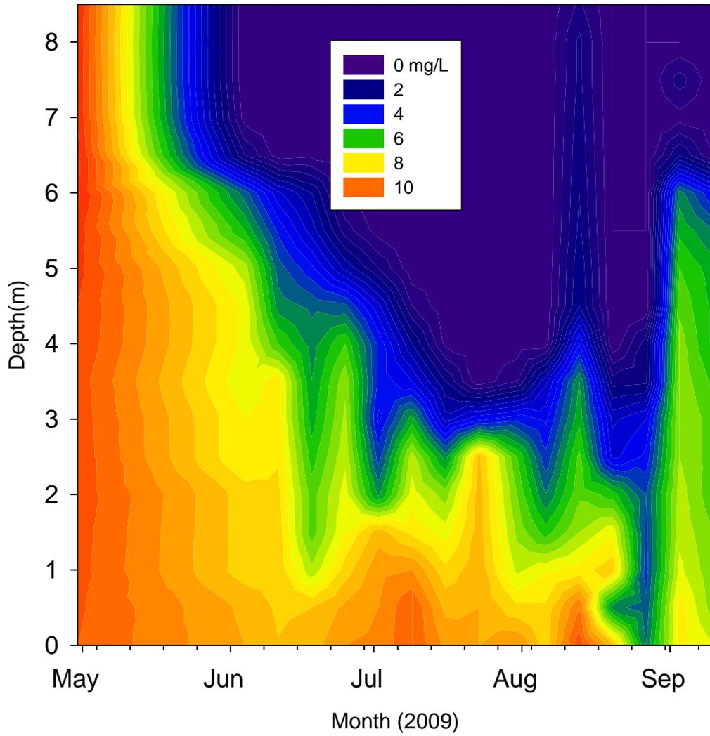
**Figure 5.** Oxygen concentrations in Irishtown Reservoir at Station 5 during the summer of 2009.
